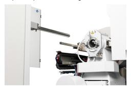
produce low NA large core optical fiber designs. Bimes MDS preform fabrication systems, combined with OptiFACT control system, are designed for optimum performance of HTS doping during active preform fabrication process. When used with Bimes FCVD systems, active preform process can be optimized for fast collapse and minimal influence of collapsing condition on preform index profile.
