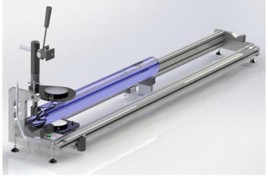
proper preform fixing, preventing vibrations and damage, as well as touch-free handling. Built-in magnifying lens and gradation on the guide rail enable exact positioning of defects relative to a chosen reference point, for process database collection and drawn fiber reference position. *NOTE: polariscope cannot determine the exact defect or inclusion size (diameter) due to cylindrical shape of the preform.*
