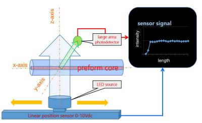
in wavelength to the active dopant in preform, as ump light source. When preform is illuminated by pump light, luminescence of the core is observed and intensity measured by a large area or integrating detector, position at right angle to the pump light direction. Pump source position (POL carriage) position and luminescence intensity are recorded by microprocessor or computer and displayed as a graph or exported as spreadsheet file.
