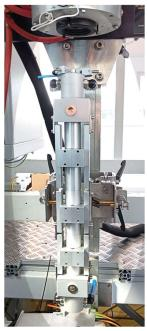
Thin carbon layer is applied to fiber surface during drawing, below the draw furnace, where the retained heat of fiber can drive a chemical vapor deposition reaction (CVD) of carbon particles to glass surface.
